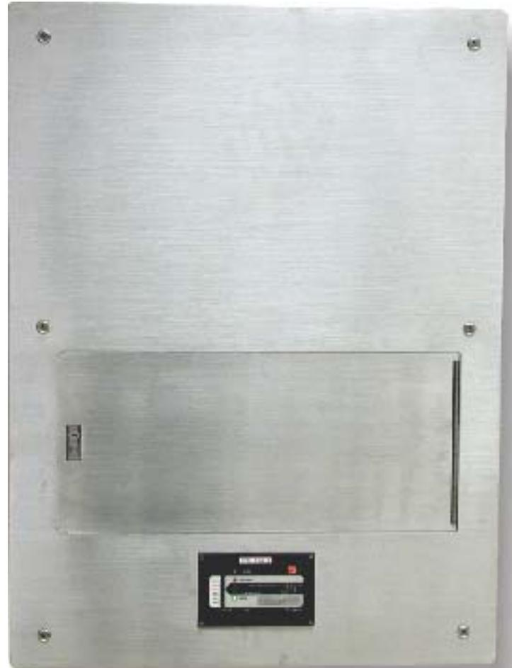
Front trim to be seamless 14 ga. 304 stainless steel with brushed finish, complete with lockable, hinged, full-access breaker compartment door. Trim to be complete with foil-backed bitumous heat and sound dampening backing in the transformer compartment.
