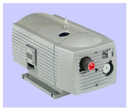
Class 1 Inc. simplex, oilless, rotary vane vacuum pump, factory assembled and tested, as follows: Model: OLRV75-RXXX1 Capacity: 2.0 SCFM @ 20" Hg [57 I / min] Menimum and uncommune 25" Hz
